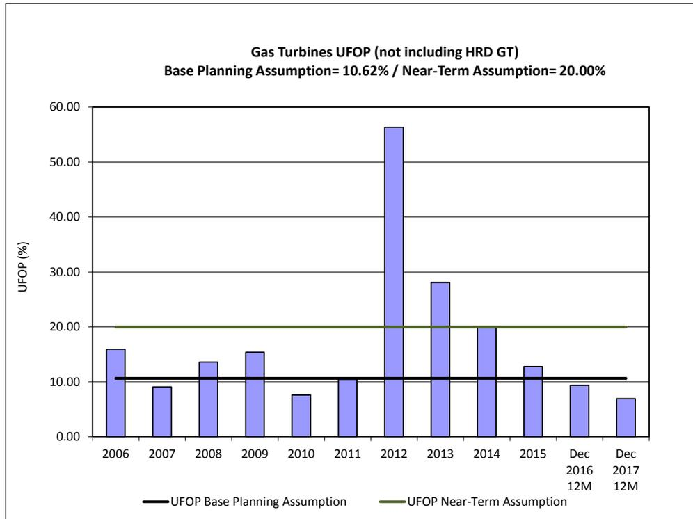
**Figure 3 Gas Turbine UFOP – HWD/HVY/SVL Units**
